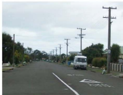
The residential good example has the same road reserve width as the poor example. The good example has more amenity - grassed berm and street trees which give it a friendly scale. The poor example is very hard and the road area is over sized for the level of use by vehicles.
