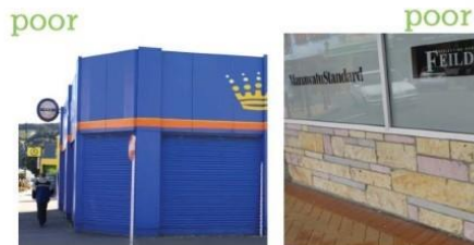
The frontage of the example above (left) has insufficient (none) window area (as well as being unsuitable given its lack of corner treatment). The example right has good window area, but this is 'blocked out' with opaque film (as well as having an inappropriate facade cladding material)
