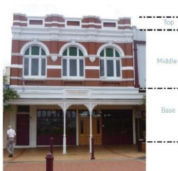
Vertical hierarchy of a base, middle and top is expressed in the size and shape of openings and balconies.
